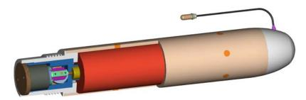
Figure 1. Warhead with vent plugs shown.
